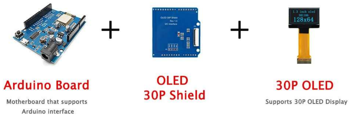
Fig. 3 System composition: main board + OLED 30P Shield + 30P OLED
