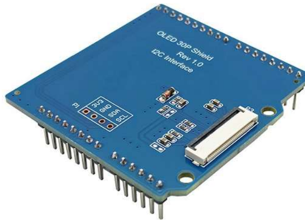
Fig. 1 OLED 30P Shield product view
